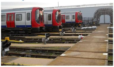
Using walk boards is the safest method of crossing the track in depots and sidings. Walk boards:
