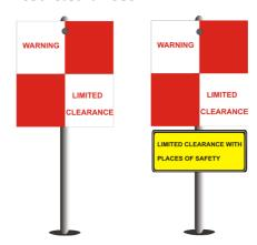
A limited clearance sign indicates places where the cess or ten foot is not a place of safety, because there is not enough room for you to stand safely between a passing train and the infrastructure.
